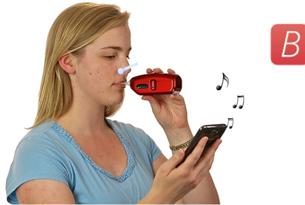
Fig 1. Breezing ® metabolic tracker and its pairing with a smartphone.
