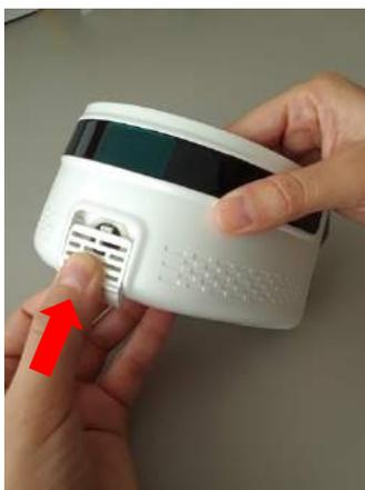
12. Close the sensor cap. The Breezing device is ready for use.
