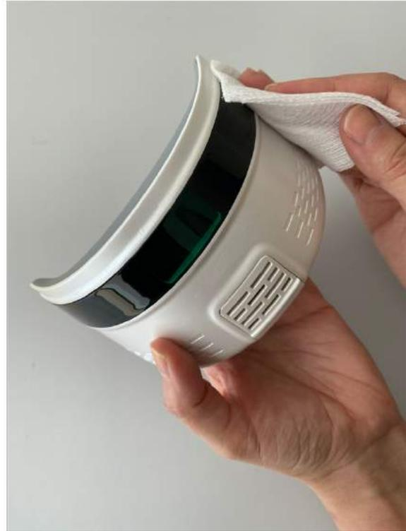
10. **Disinfection of the air channel and grate:** grate is to be immersed in the 70% IPA solution for at least 60 seconds and allowed to thoroughly dry. Afterward, use a 70% IPA-soaked polyethylene swab to wipe firmly and thoroughly the entire air channel and grate. Ensure the entire surface has been soaked with 70% IPA.
